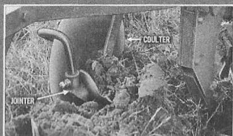
JOINTER SLICES AND TURNS STRIP OF SOIL AT THE SIDE OF FURROW SLICE FOR BETTER TRASH COVERAGE
